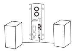
Connect an auxiliary source to the audio input jacks in rear panel.
